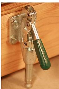
**Wagon locks** are used to keep wagons from moving while actors are on them. They are mounted on the upstage side of wagons so the audience can't see them. (These devices aren't brakes. They simply lift the wagon slightly off the ground so it won't roll.) The lever on this device can be pushed into a locked position with a hand or foot.
